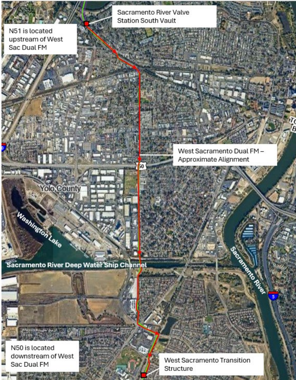
Figure 1: West Sacramento Dual Force Main Alignment
